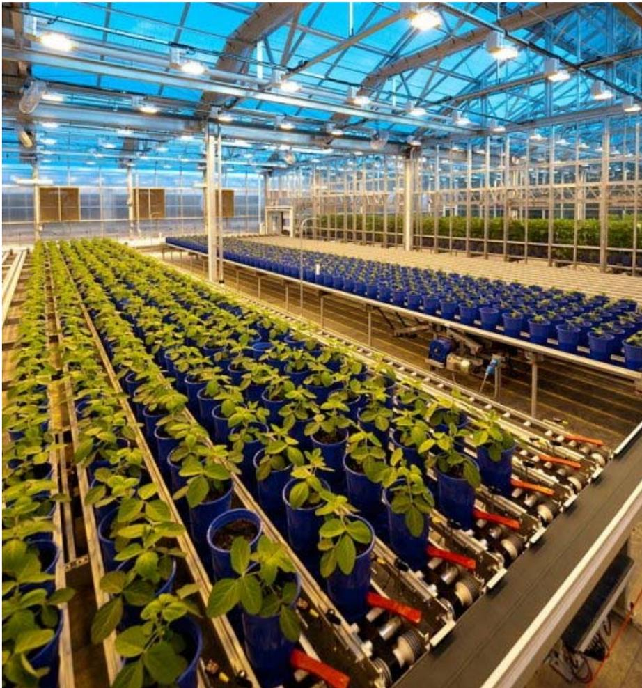
Soybeans in Automated Greenhouse Genetically modified soybean plants grow at Monsanto's automated greenhouse in Raleigh, N.C. The greenhouse has conveyor belts to move plants around for watering, weighing, and pictures, so scientists can monitor their health without ever having to handle them. Courtesy Monsanto
